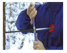
Press the borer tip to the stem in a straight 90° angle. To get an accurate age of any tree, the rings should be counted near the tree base or the ground. Turn the handle and press the borer firmly to the stem and turn at the same time. It is important to keep a straight angle and to avoid putting weight onto the handle while drilling. It is recommended to use a borer starter to get a straight angle when drilling into the wood.
